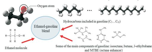
could be fully biodegradable and renewable [16, 22]. Another advantage is that it has high octane number in comparison to gasoline. Ethanol very easy absorb water which make it problematic to storage. Moreover, it has a higher density and viscosity than gasoline [22, 29, 31] and is generally more penetrative
