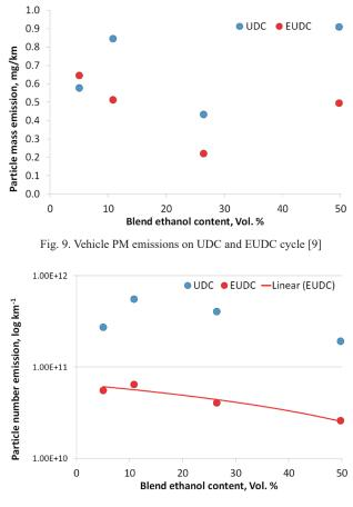
Fig. 10. Vehicle PN emissions on UDC and EUDC cycle [9]
