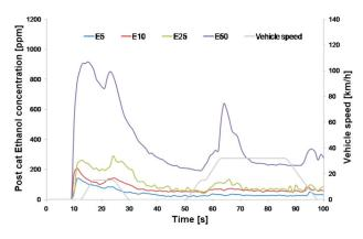
Fig. 11. Pre cat ethanol concentrations for various blends over the first 100 seconds of the NEDC (source: BOSMAL data – see [9] for commentary)
